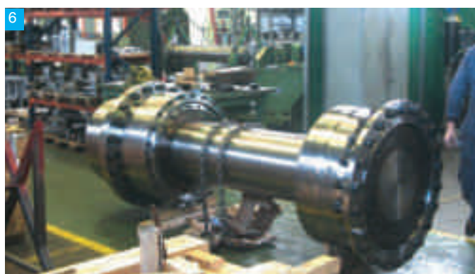
7 Special MTGX-420 with spacer & angular adjustment positioning.
